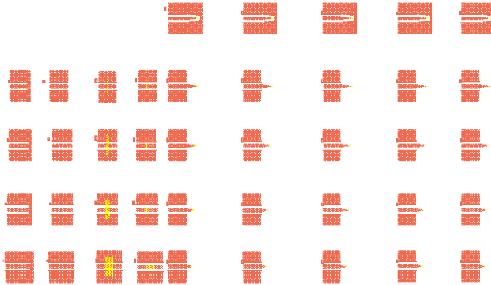
Figure 5 : Generic layout for CNT-based monopole in CPW technology (HR Si and quartz substrate)
